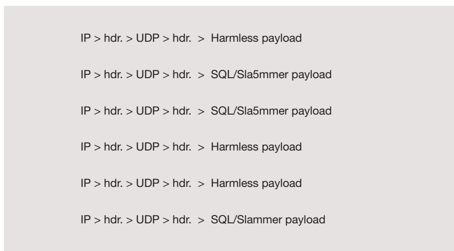
Figure X An additional differentiating characteristic of the SQL/Slammer worm was that all packets had the same length. Legitimate packets were unlikely to match this size, and therefore, a fine-grained signature that took the length into account was able to identify only the worm packets with high accuracy.
